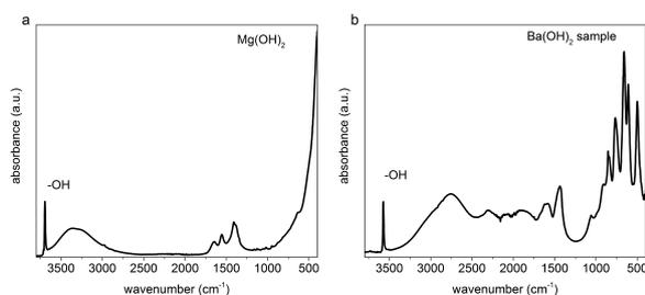
FIGURE 2. a) FTIR spectrum of  $\text{Mg}(\text{OH})_2$  sample; b) FTIR spectrum of  $\text{Ba}(\text{OH})_2$  sample.
