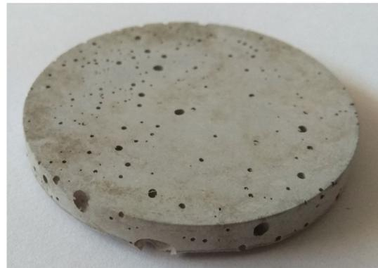
FIGURE 1. Concrete specimen (diameter 55 mm, height 5 mm).
