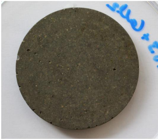
FIGURE 9. Surface of the specimen placed in solution of bacteria in 253 media in 2%  $\text{CaCl}_2$  solution.
