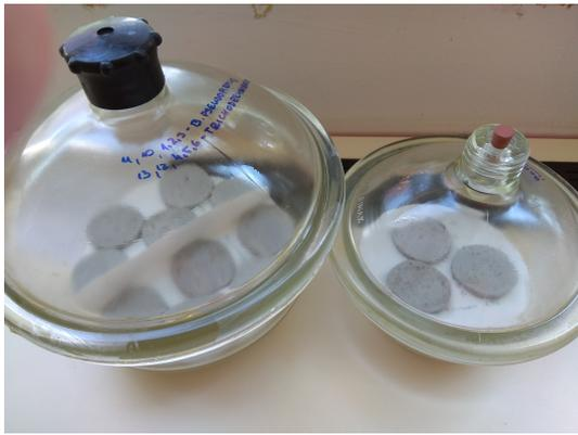
FIGURE 6. Concrete specimens in desiccators.
