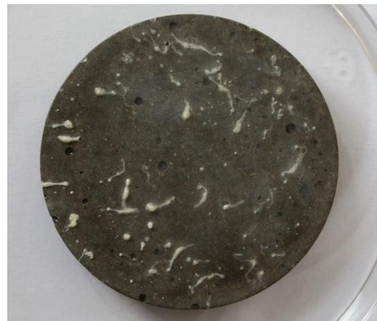
FIGURE 11. Surface of the specimen placed in solution of bacteria in 253 media.
