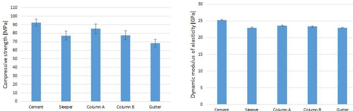
FIGURE 3. Mechanical properties of tested composites, compressive strength – left, dynamic modulus of elasticity – right.
