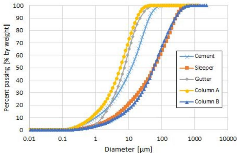
FIGURE 1. Grain curves for cement and individual samples of recyclates.
