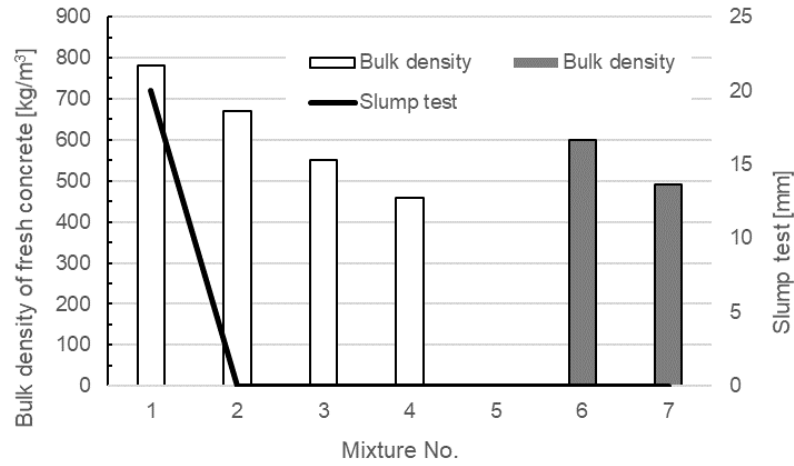
FIGURE 2. Bulk density and consistency of fresh lightweight concrete.
