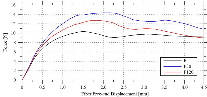
FIGURE 1. Pull-out behavior of reference and modified fibers.
