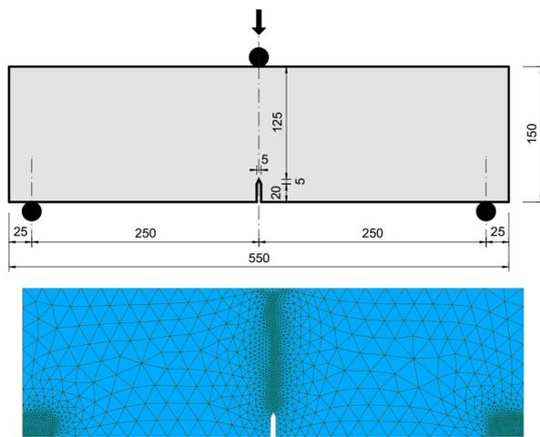
FIGURE 2. Geometry of FRC specimen (top) and mesh of computational model (bottom).
