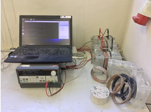
FIGURE 1. An electromigration setup used for accelerated chloride penetration/extraction tests.
