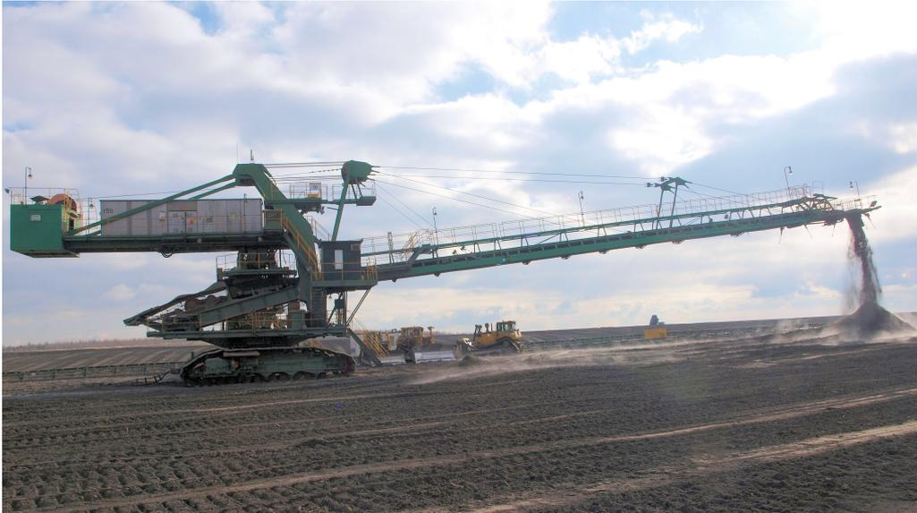
FIGURE 1. Stacking the deposit material in the technical reclamation area using a belt stacker.
