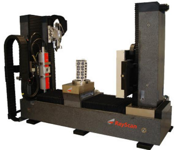
FIGURE 3. Image of the RayScan 250E system with dual sources on the left and flat panel detector on the right. An exemplary specimen is positioned on the rotary stage in-between.
