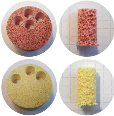
FIGURE 1. Examples of CaP (red) and CaC (yellow) foams as casted (left) and the final specimens after hollow-core drilling (right).
