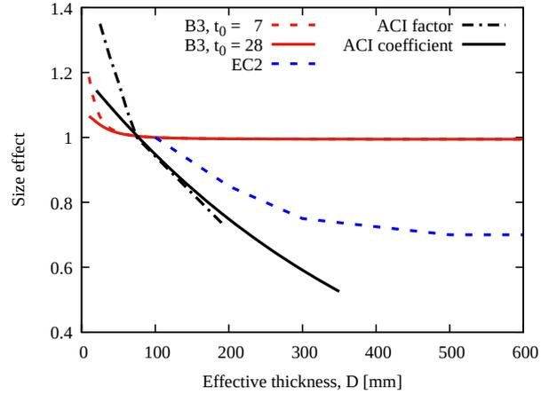
FIGURE 1. Size effect on ultimate drying shrinkage evaluated according to selected design codes and prediction models.
