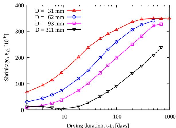
FIGURE 2. The experiment of L’Hermite (data adapted from [16]) shows incomplete drying shrinkage of the largest specimen with  $D = 311$  mm. Such measurements were not discarded but are denoted by empty symbols in Fig. 4.
