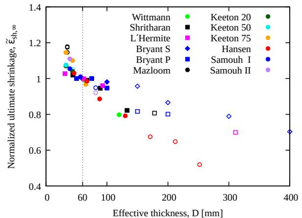
FIGURE 4. Influence of the effective thickness on the normalized experimentally measured ultimate shrinkage strain. The strain is normalized with respect to the value corresponding to  $D = 60$  mm, empty symbols mark the last data points in prematurely terminated experiments.
