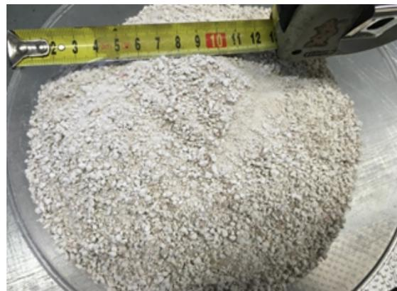
FIGURE 4. Milled gypsum before sorting and without paper.
