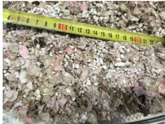
FIGURE 3. Crushed plaster boards with paper.
