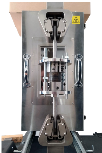
FIGURE 2. Construction for pull-off tests fixed in loading frame. In the middle, there is a sandwiched specimen placed.
