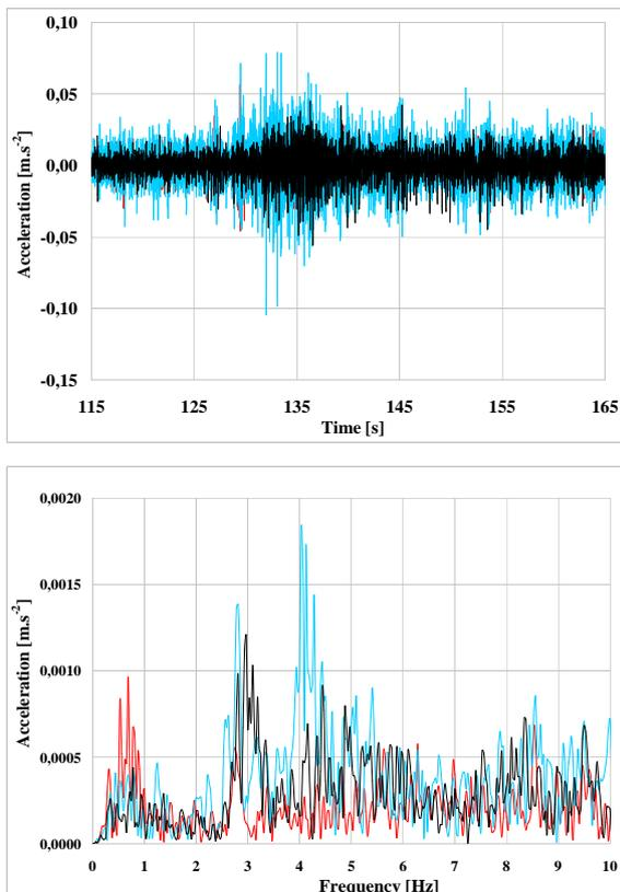
FIGURE 10. IBB, dynamic response of the stand – Bouncing – axes  $z$  [3].
