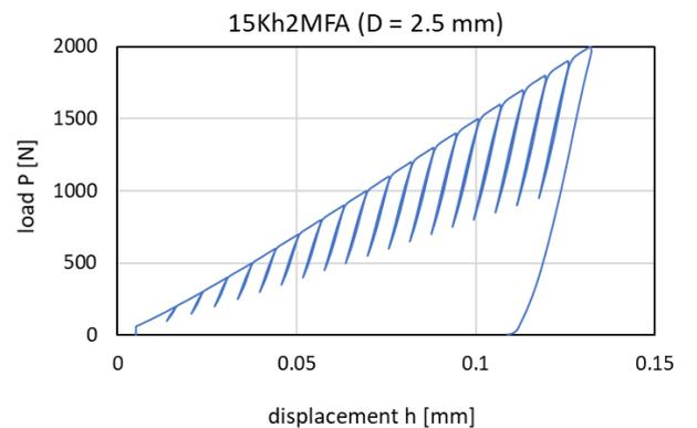
FIGURE 1. ABI test load - displacement curve for 15Kh2MFA steel.
