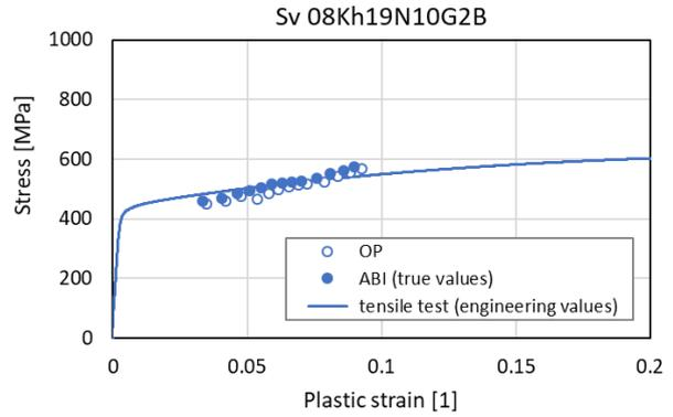
FIGURE 5. True stress/plastic strain curves for Sv 08Kh19N10G2B steel obtained by various techniques.
