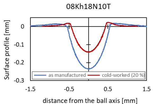
FIGURE 9. Cross-sectional profile of the spherical indent in undeformed and cold deformed 08Kh18N10T steel.
