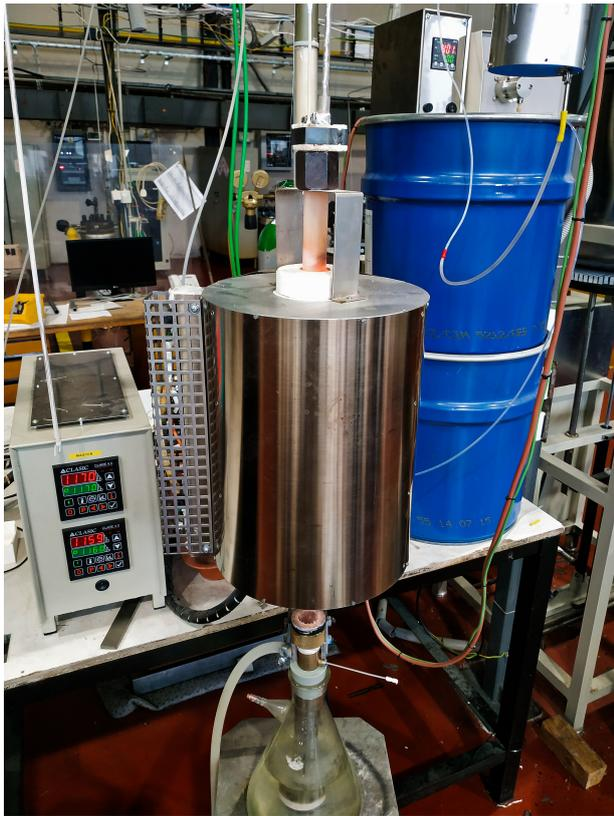
FIGURE 4. The apparatus for high-temperature oxidation.
