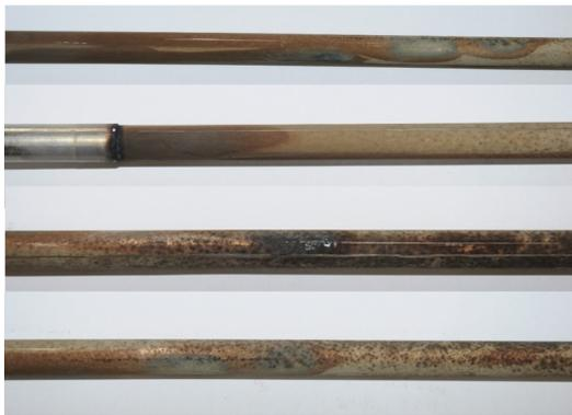
FIGURE 7. Detail of the test section with post glowing spots
