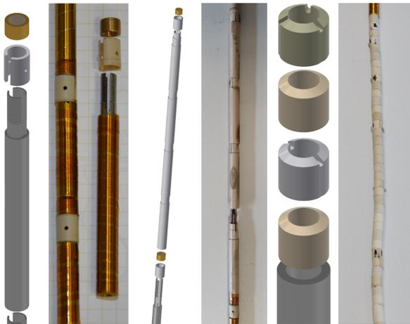
FIGURE 3. From left to the top is a design and its actual photography of the first, the second and the third version of measurement probe.
