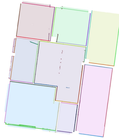
FIGURE 4. Vertical plane segmentation (top view). Door planes are segmented as they cover sufficient area, also notice the noise around outer windows and in the center room.
