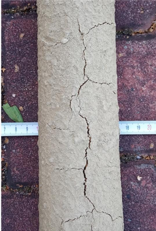
FIGURE 8. The state of the tube shape surface of the micropile after being pulled out of the ground.
