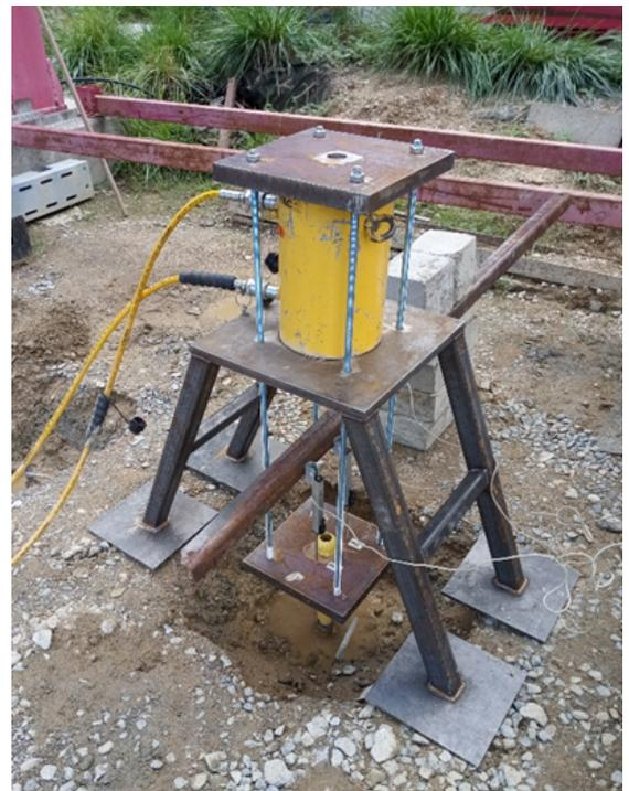
FIGURE 7. Installation of the traction rig at micropile traction load test.
