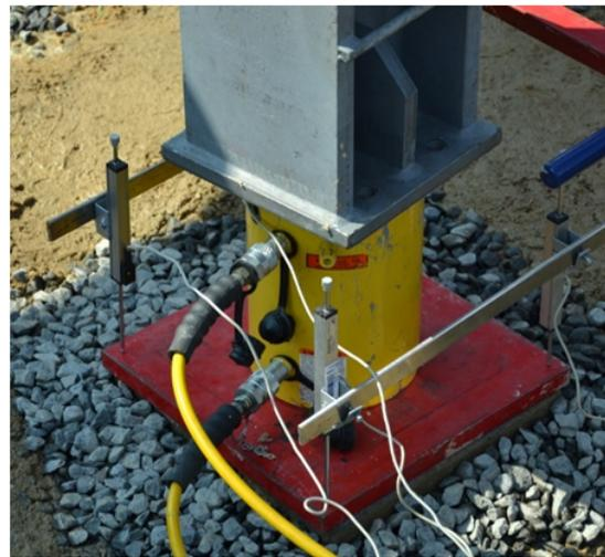
FIGURE 5. Installation of hydraulic press on the micropile at the micropile compression load test.
