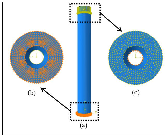
FIGURE 3. Circular hollow unconfined RC column modeled in ABAQUS FEA; (a) Front view (b) bottom plan view showing support boundary condition (c) Upper plan view showing full axial load imposed on top of the column.
