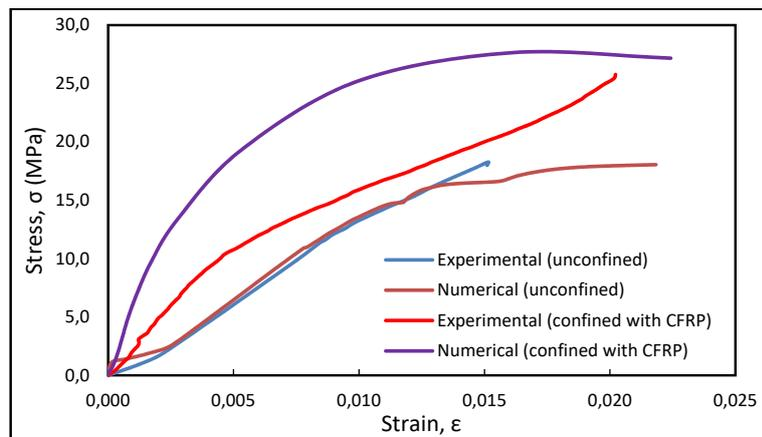
FIGURE 9. Validation process stress-strain relationship of circular hollow unconfined and confined RC column with CFRP under full axial load.
