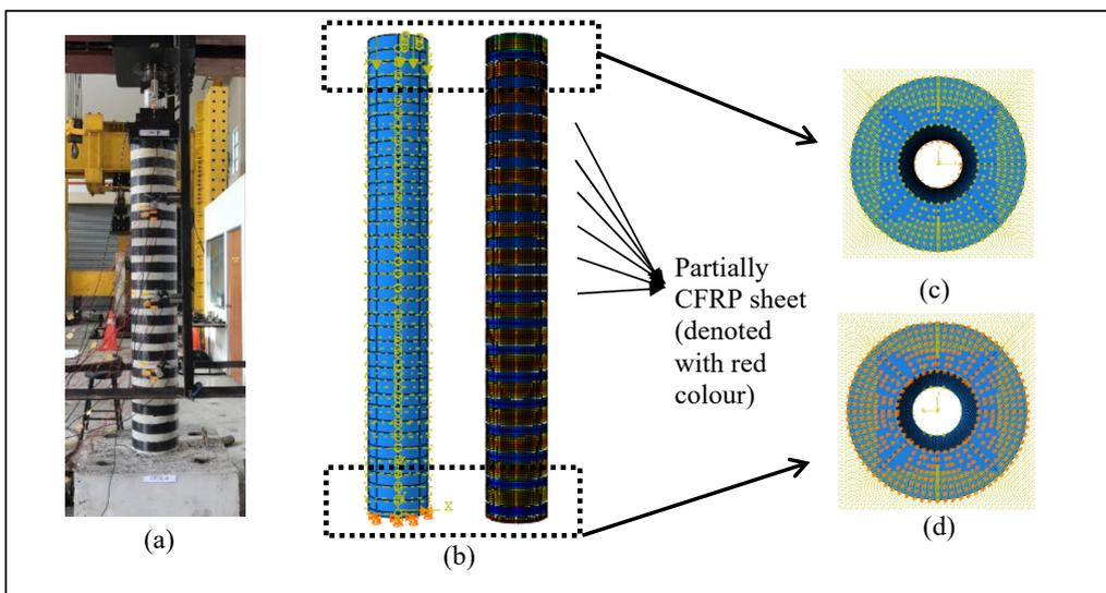
FIGURE 4. Circular hollow confined RC column strengthened with CFRP sheet experimental set-up and modeled in ABAQUS FEA; (a) Front view from experimental set-up (b) Front view (c) Upper plan view showing full axial load imposed on top of the column (d) bottom plan view showing support boundary condition.
