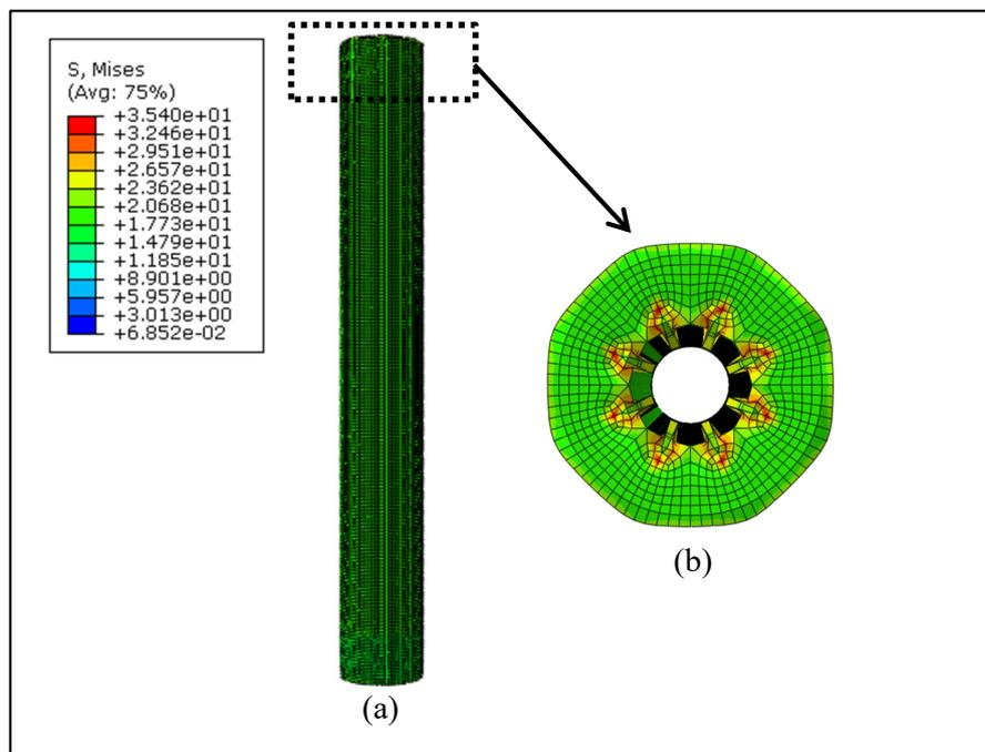
FIGURE 7. Predicted von Mises stress of circular hollow unconfined RC column (at the end of simulation analysis); (a) Front view (b) Upper plan view showing failure behavior on top of the column.
