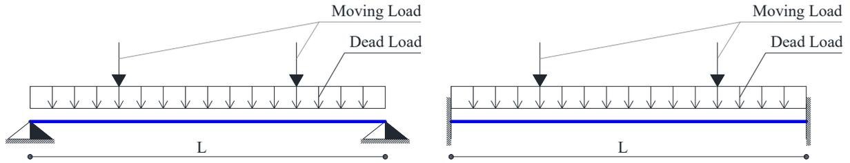
FIGURE 4. Different constraint conditions for the secondary beams.
