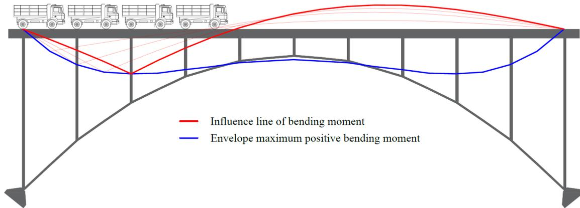
FIGURE 3. Influence line of bending moment and position of the moving loads able to maximize the positive bending moment.
