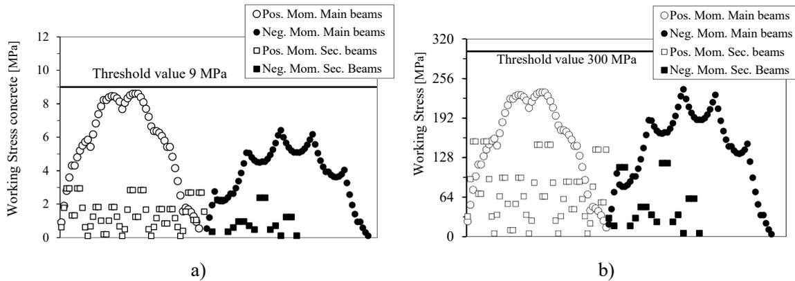
FIGURE 8. Structural verifications for bending moment in the beams: a) compressed concrete, b) steel reinforcement in tension.
