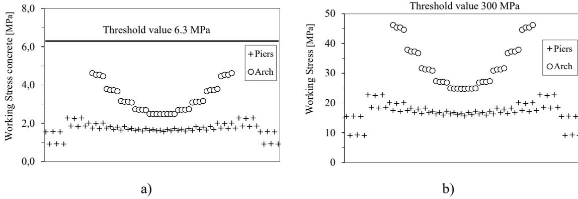
FIGURE 7. Structural verifications of compression stresses in the arch and the piers: a) compressed concrete; b) compressed steel reinforcement.
