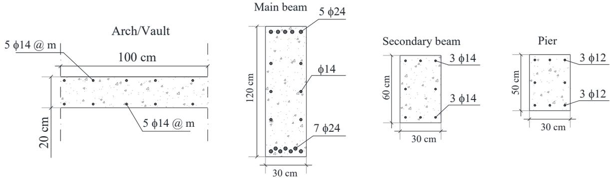
FIGURE 5. Details of cross section and steel reinforcement of different structural elements.
