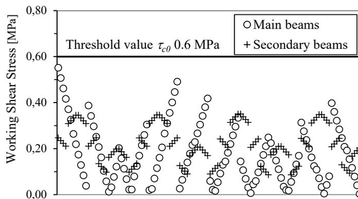
FIGURE 9. Structural verifications for shear in the beams..
