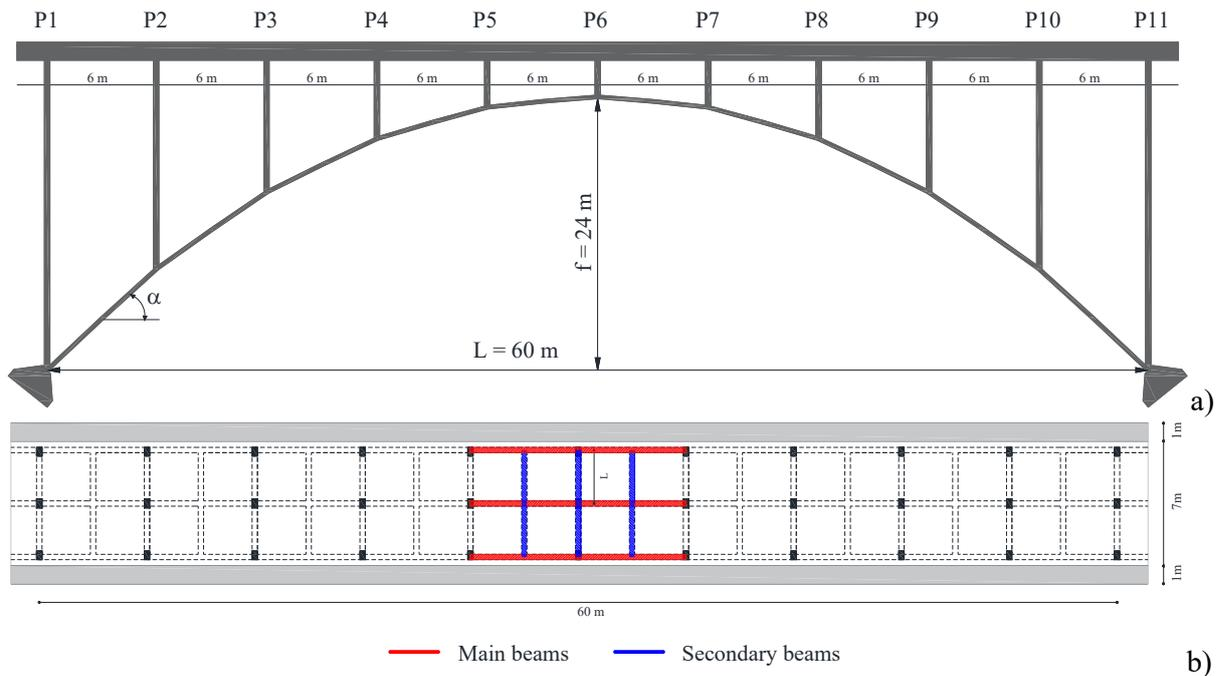
FIGURE 2. a) Longitudinal view of the deck arch bridge assumed as case study; b) Plan view of the deck.
