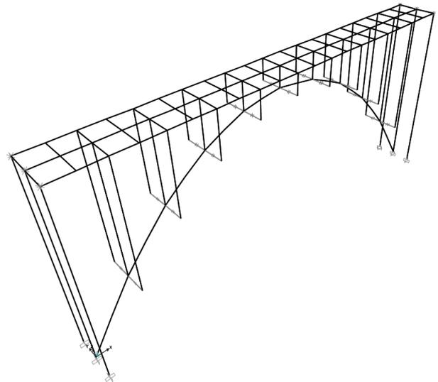
FIGURE 6. 3D FE model of the RC deck arch bridge assumed as case study.
