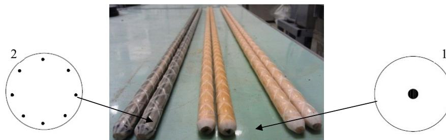
FIGURE 1. Experimental samples of FRPR; CF location.
