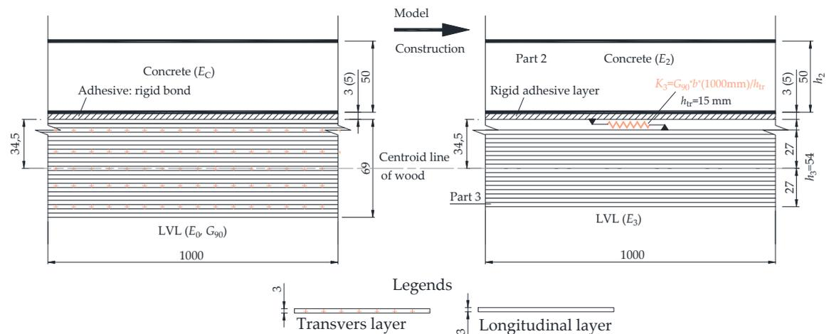
(b) Concrete-LVL composite decks
