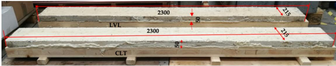
FIGURE 1. Dimensions of fabricated TCC decks.
