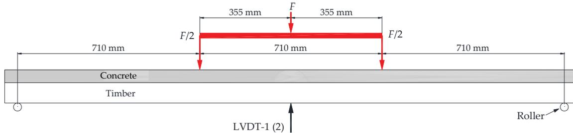
FIGURE 2. Setup of 4-point bending test.
