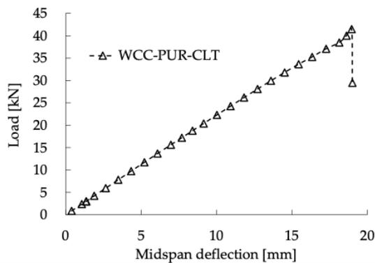
FIGURE 3. Load vs. displacement responses of WCC-PUR-CLT at mid-span.
