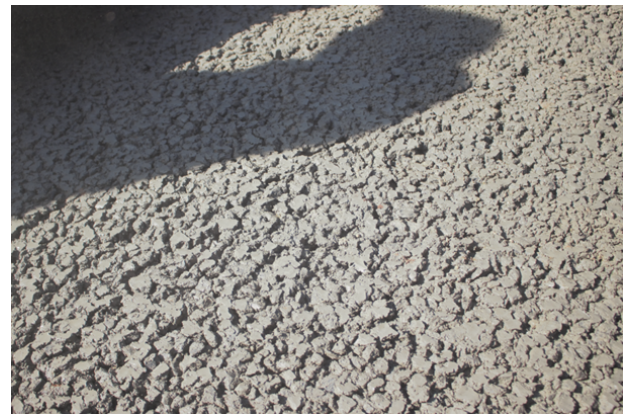
FIGURE 5. Detail of pervious concrete surface with D_{max} = 16 mm.
