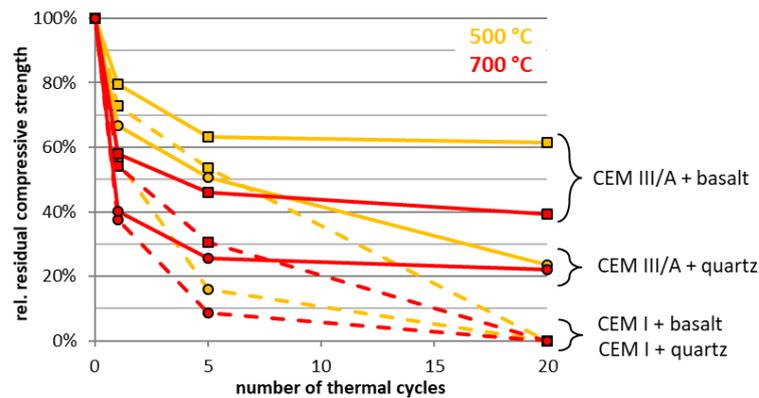
FIGURE 4. Combined effects of type of cement and aggregate on the residual compressive strength after cyclic heating with maximum temperatures of 500 °C and 700 °C.
