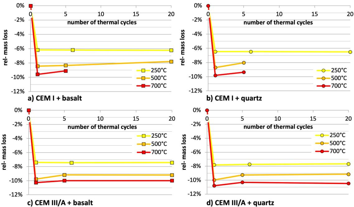
FIGURE 6. Mass loss induced by cyclic heating for all tested concretes.
