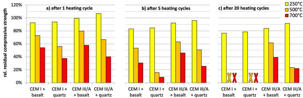
FIGURE 2. Residual compressive strength after 1 heating cycle (a), 5 heating cycles (b) and 20 heating cycles (c). Crosses (X) denote untestable mixtures due to complete degradation.
