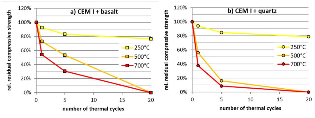
FIGURE 3. Residual compressive strength for concrete containing CEM I and basalt (a) and quartz (b).
