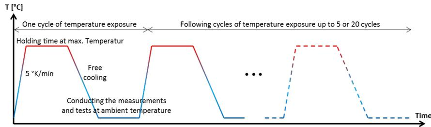
FIGURE 1. Sketch of the heating program, each complete cycle having a duration of 24 h.
