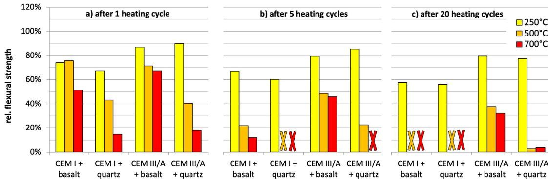
FIGURE 5. Residual flexural strength of the concretes after 1 cycle (a), 5 cycles (b) and 20 cycles (c).
