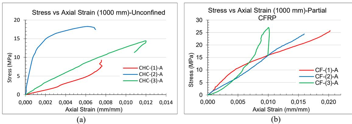
FIGURE 6. Stress vs Axial Strain; (a) Unconfined CHRCC (b) Partial CFRP CHRCC.
