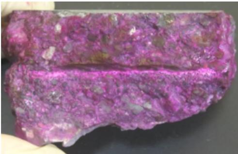
FIGURE 18. Observation results of steel mark in concrete test piece after neutralization test.
