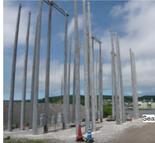
FIGURE 7. Exposure test of "CP350" utility poles at the Muroran test site in Japan (started in July 2013).
