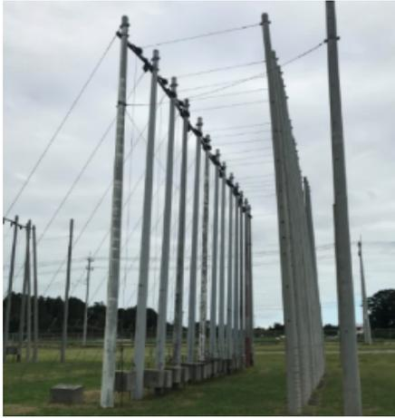
FIGURE 6. Exposure test of "CP500" utility poles at the Choshi test site in Japan (started in August 2010).
