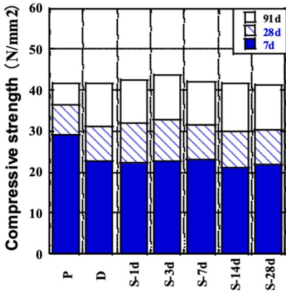
FIGURE 7. 20-in compressive strength for each age of A-ash S.
