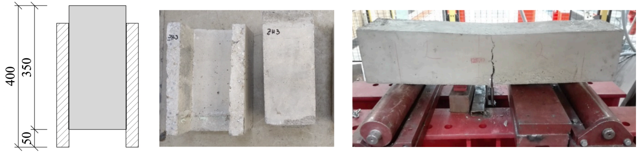
FIGURE 3. Push test and 3-point bending test, a) dimension of a push test, b) push test after the loading, c) sample after the 3-point bending test.
