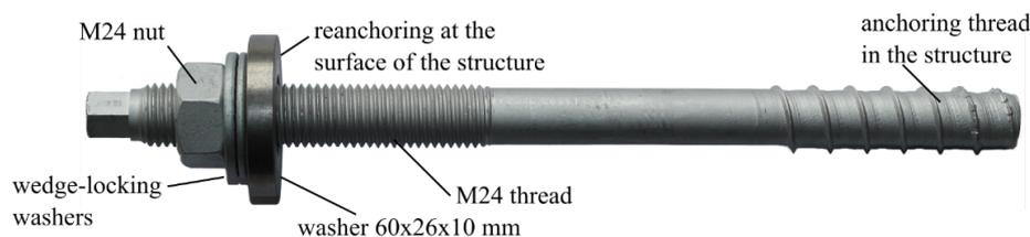
FIGURE 1. Concrete Screw Anchor with anchoring thread which creates a form-locked connection and the re-anchoring at the concrete surface of the structure.
