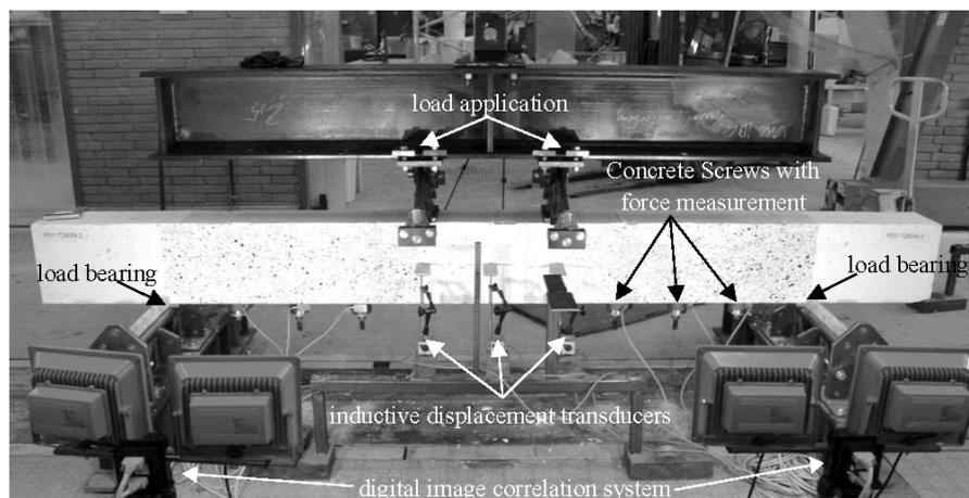
FIGURE 2. Test setup and measuring systems of the shear tests with concrete screw anchors at the University of Innsbruck.
