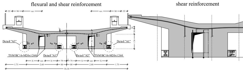
FIGURE 4. Additional flexural reinforcement on both sides of the hollow box girder and additional shear reinforcement drilled through the hollow box.
