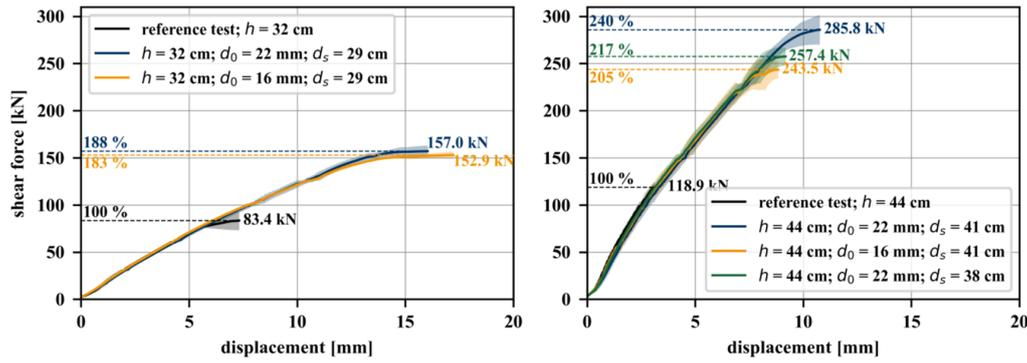
FIGURE 3. Test results of concrete test girders with heights of 320 mm and 440 mm and with concrete screws of different diameters  $d_0$  (22 mm and 16 mm) and different installation depth  $d_s$ .
