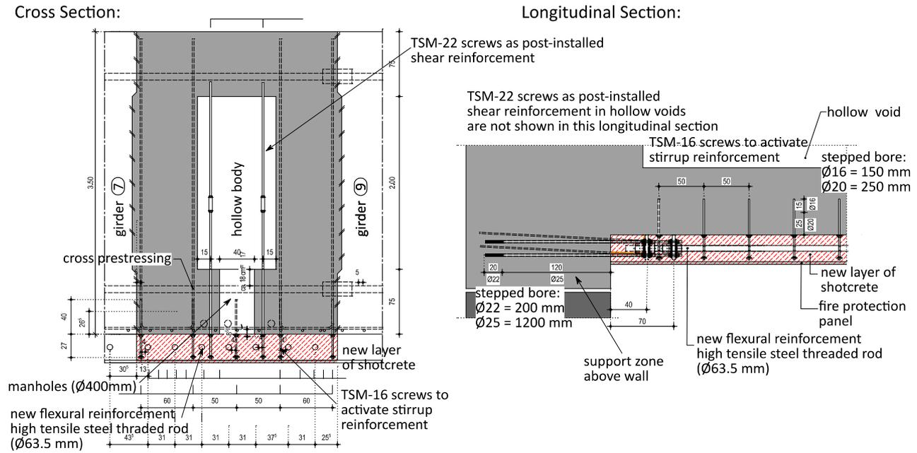
FIGURE 6. Planned shear and flexural reinforcement by the use of concrete screw anchors as shear reinforcement and threaded rods of high tensile steel as new flexural reinforcement.
