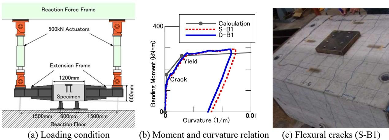
FIGURE 2. Development of initial flexural cracks.
