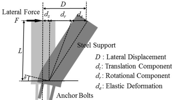
FIGURE 7. Components in lateral displacement.
