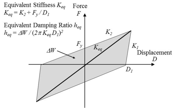
FIGURE 8. Equivalent stiffness and damping ratio.
