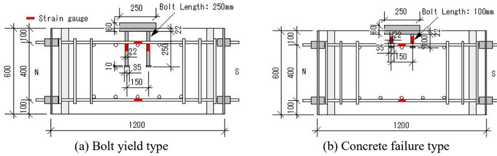
FIGURE 1. Test specimens (Unit: mm).
