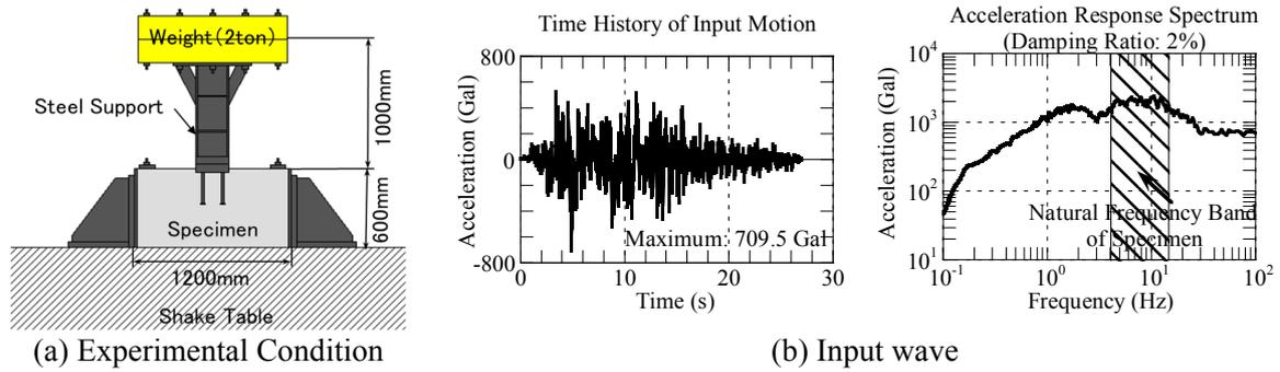
FIGURE 4. Loading conditions in the shake table test.
