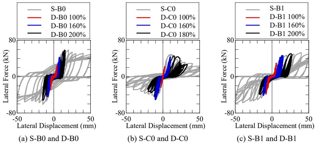
FIGURE 5. Lateral force and lateral displacement relationships based on the static and dynamic tests.
