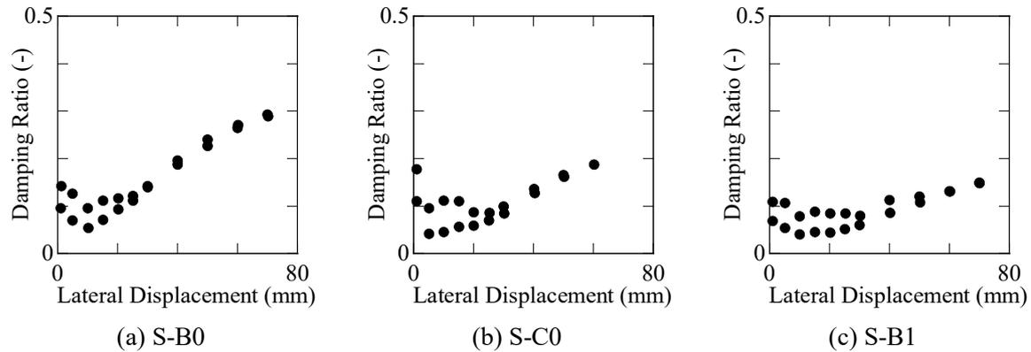
FIGURE 11. Equivalent damping ratios based on the static loading tests.
