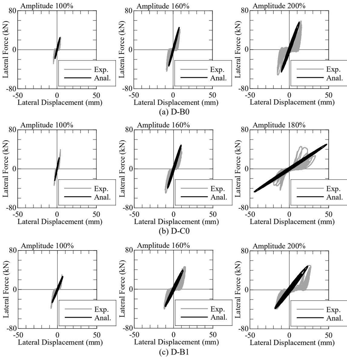
FIGURE 12. Analytical results based on the linear model.
