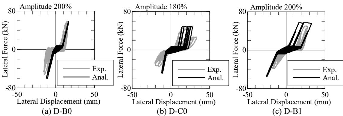
FIGURE 13. Analytical results based on the nonlinear model.
