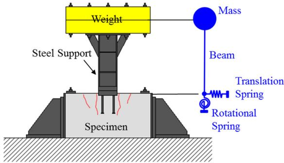
FIGURE 6. Analytical idealization for the specimen.
