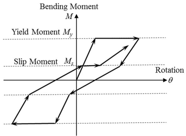
FIGURE 9. Nonlinear model for rotational spring [6].
