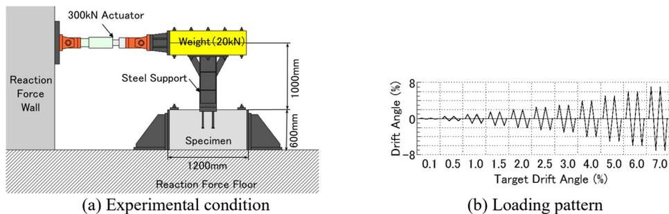
FIGURE 3. Loading conditions in the static loading test.
