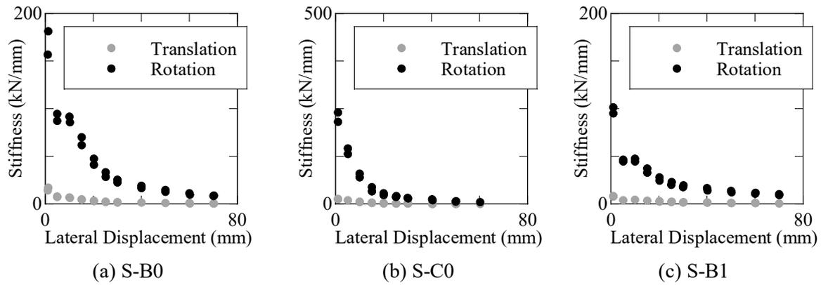
FIGURE 10. Equivalent stiffness based on the static loading tests.
