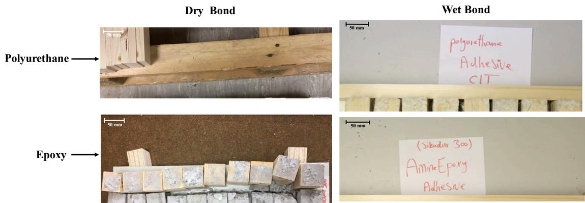
FIGURE 6. Fracture surfaces of timber-prefabricated concrete and timber-cast-in-situ concrete glued with polyurethane and epoxy adhesives.
