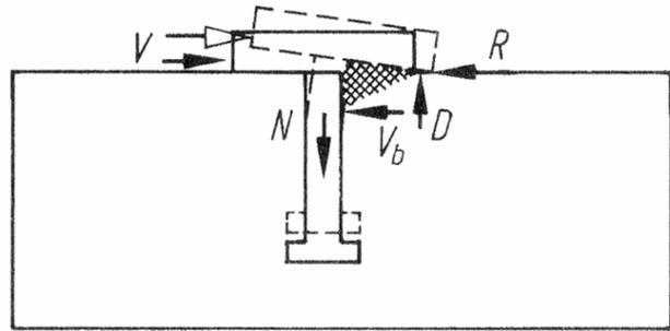
FIGURE 7. Supporting mechanism of a head bolt anchorage due to shear load (Eligehausen, Mallée & Silva 2006)
