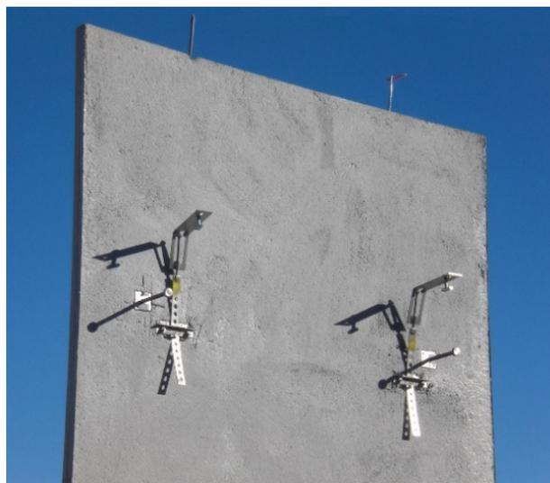
FIGURE 3. Storey-high façade element with new fixing system for carbon reinforced concrete.
