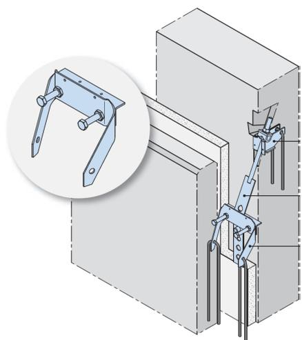
FIGURE 10. Fixing system for façade panels.
