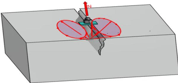
FIGURE 6. Stress distribution in cracked concrete due to splitting.
