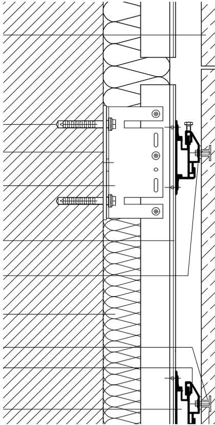
FIGURE 1. Principle cross-section curtain wall façade.
