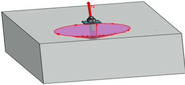
FIGURE 5. Stress distribution in uncracked concrete.
