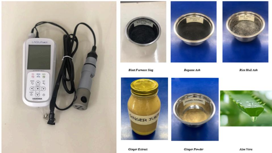
FIGURE 2. DO meter and sample candidate materials.
