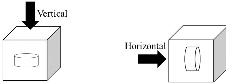
FIGURE 2. Air permeability test.
