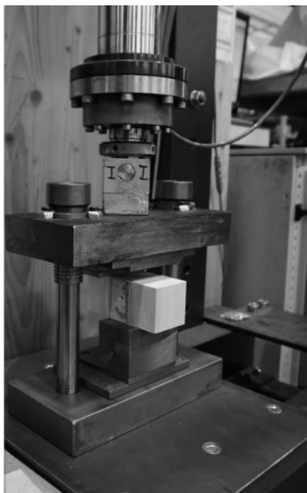
FIGURE 5. Experimental test setup for shear experiments [5].
