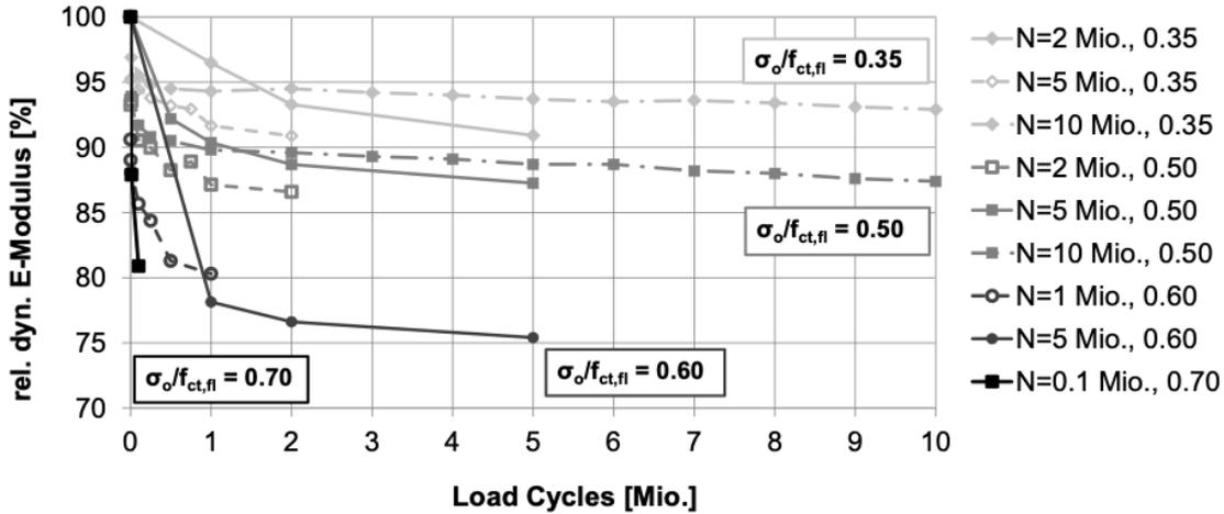
FIGURE 3. Decrease of the rel. dyn. E-Modulus of beams after 5 million load cycles and at different stress-ratios.
