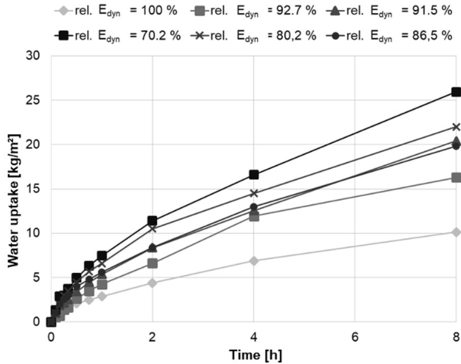
FIGURE 4. Water uptake in concrete with different relative dynamic E-Modulus.
