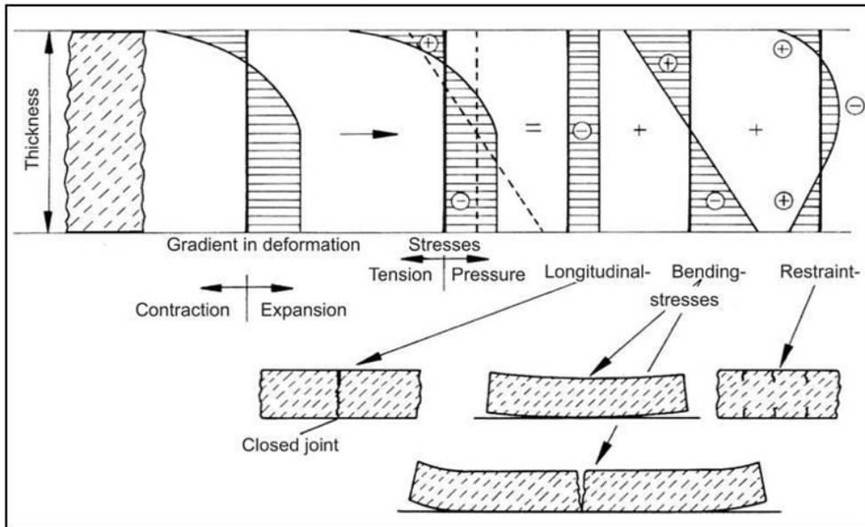
FIGURE 1. Stresses and cracks in concrete pavements due to negative gradients of deformation [7].
