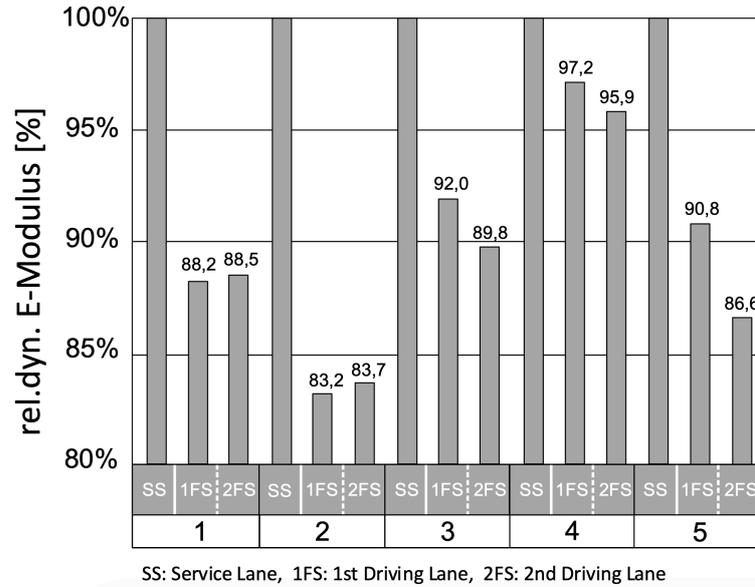
FIGURE 2. Relative Dynamic E-Modulus of the service lane (SS) and the driving lanes (1.FS and 2. FS) [13].
