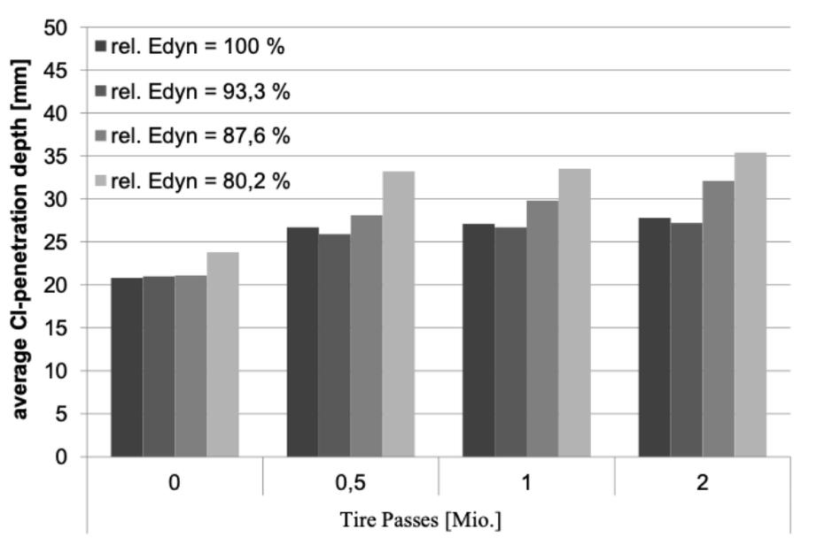
FIGURE 5. Average chloride penetration depth dependent on the number of tire passes and microstructural damage
