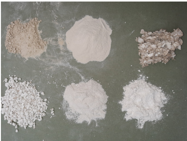
FIGURE 3. Raw materials and outputs from the recycled process.
