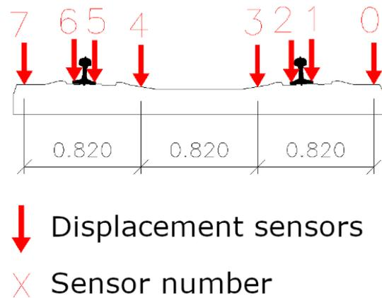
FIGURE 3. Schematic of sensor placement [3].
