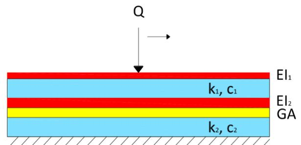
FIGURE 1. Schematic of the two-layer model on Pasternak foundation.
