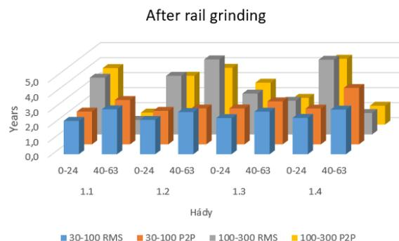
FIGURE 5. Number of years needed to reach the wave defect progression of the same level as before the rail grinding.
