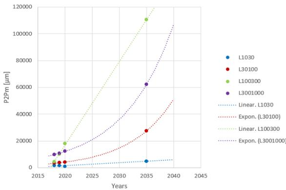
FIGURE 6. Wave defects development prediction based on the previous measurements done by the Track recording car.
