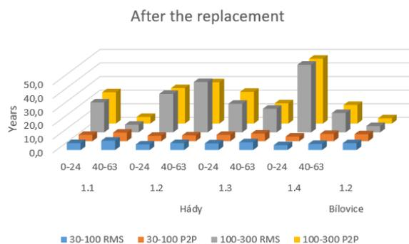
FIGURE 4. Number of years needed to reach the wave defect progression of the same level as before the rails replacement.
