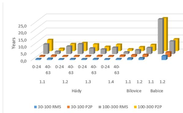
FIGURE 7. Timeframe needed for the defect progression according to Table 17 (ČSN 13231-3:2006 [6]).
