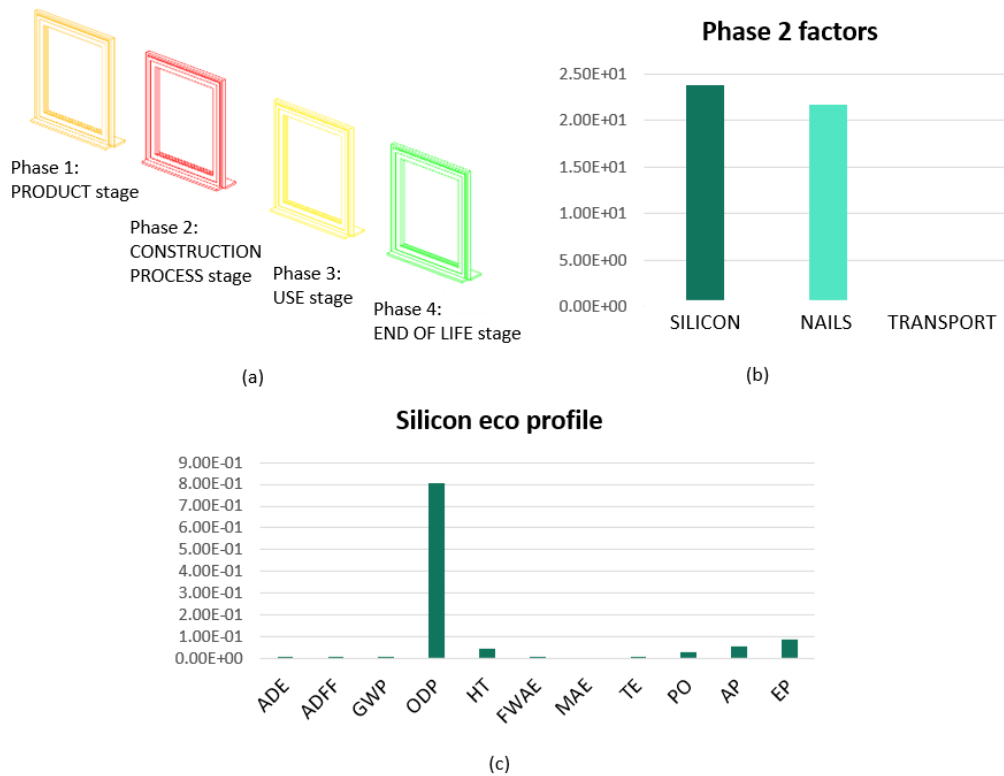
FIGURE 3. Results visualization options: (a) colour variation of the four life cycle phases, considering the impact category “Human Toxicity” (HT), (b) bar diagram of the environmental impacts factor of the installation phase and (c) bar diagram of the silicon eco-profile.
