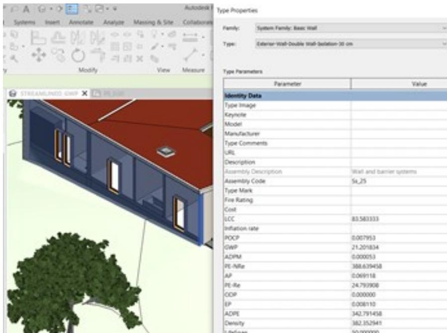
FIGURE 5. Environmental Impacts incorporated in shared parameters of a wall in Revit.
