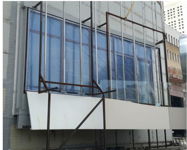
FIGURE 2. Air permeability test on mock-up 02.
