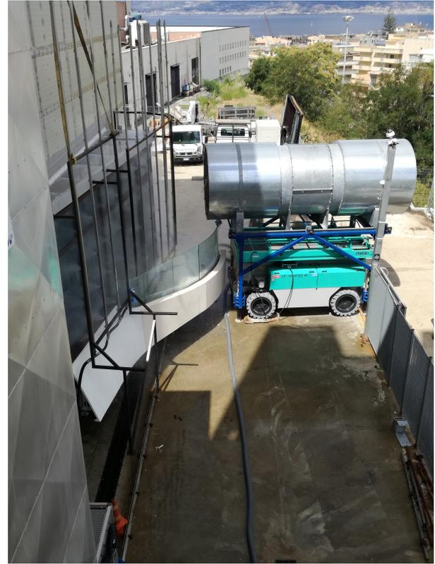
FIGURE 4. Hurricane test on mock-up 02.
