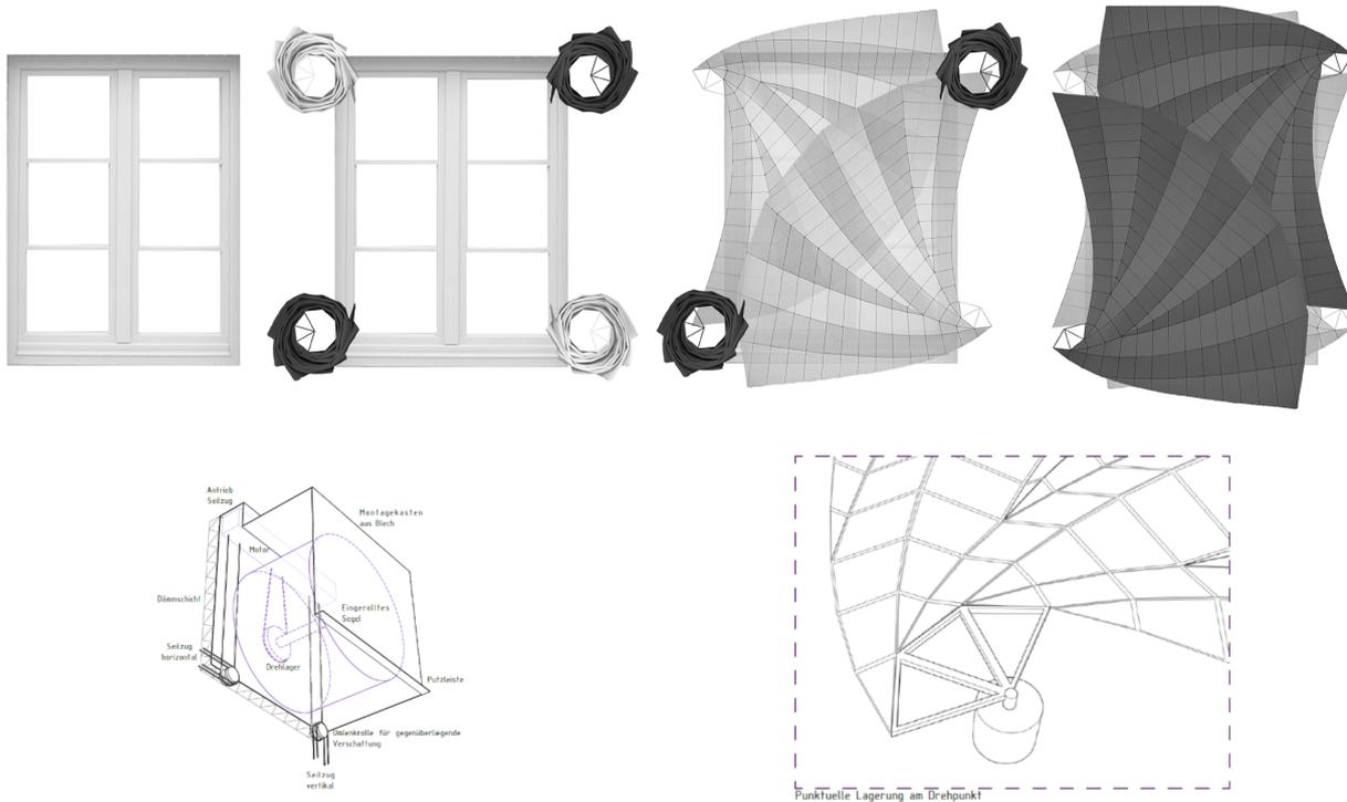
FIGURE 2. Project 2: Whirlshade: Upper Row: Installation and opening sequence; Lower Row left: Box with mechanics (pulleys, motorization); Lower Row right: principle construction of the foldable sail.
