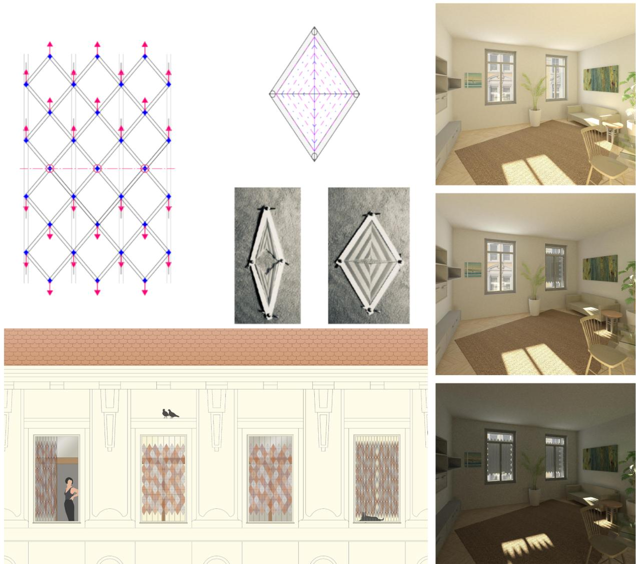
FIGURE 1. Project 1: Rutatus-Blende: Upper left: functional principle, Lower left: Façade view by integration in a Gründerzeit façade, sequence on the right: Shading effect / sun penetration reduction (rendering).
