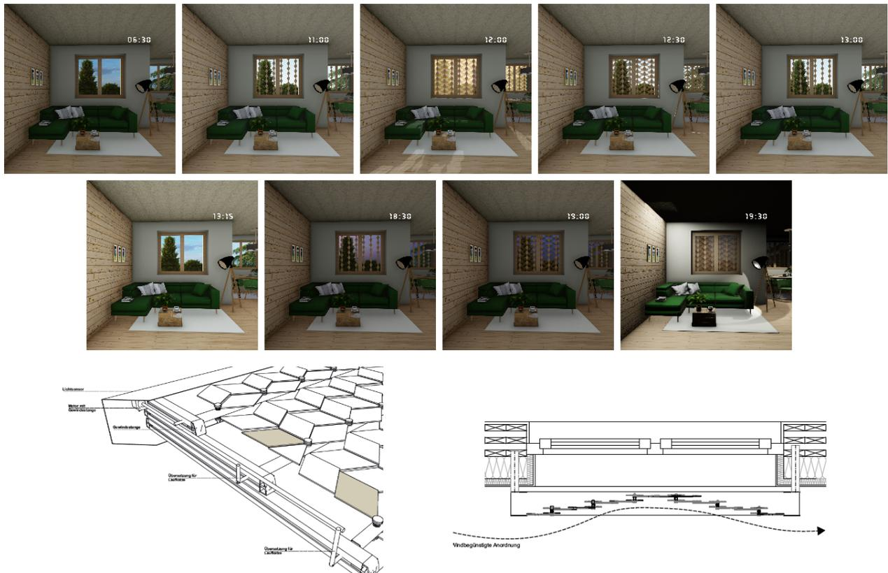
FIGURE 3. Project 3: Sonnensterne: Upper rows: Sequence of different states of deployment; Lower Row: Isometry and horizontal section of the technical principle of Sonnensterne.
