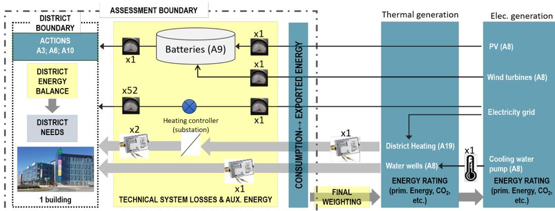
FIGURE 5. Monitoring example for the Viiki building in Helsinki.
