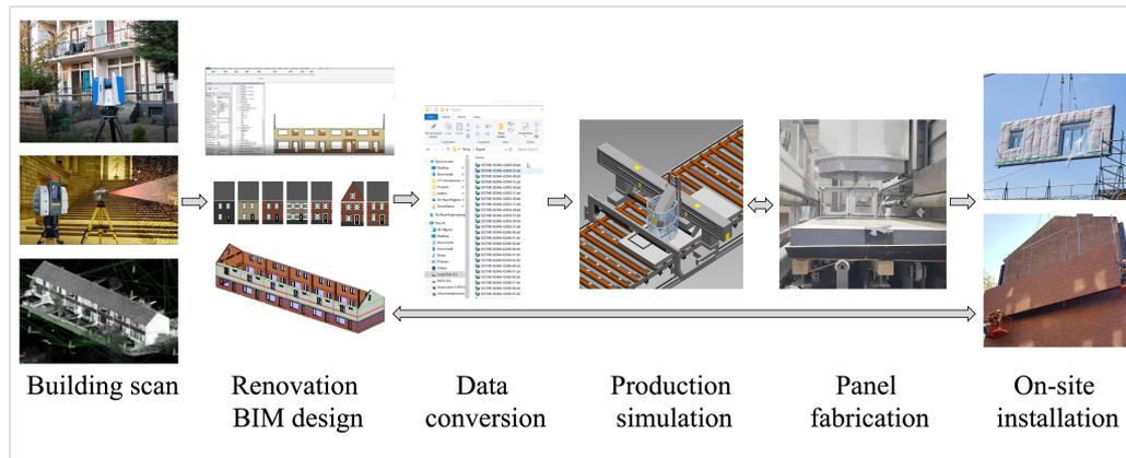
FIGURE 3. Future INDU-ZERO construction supply chain process overview.
