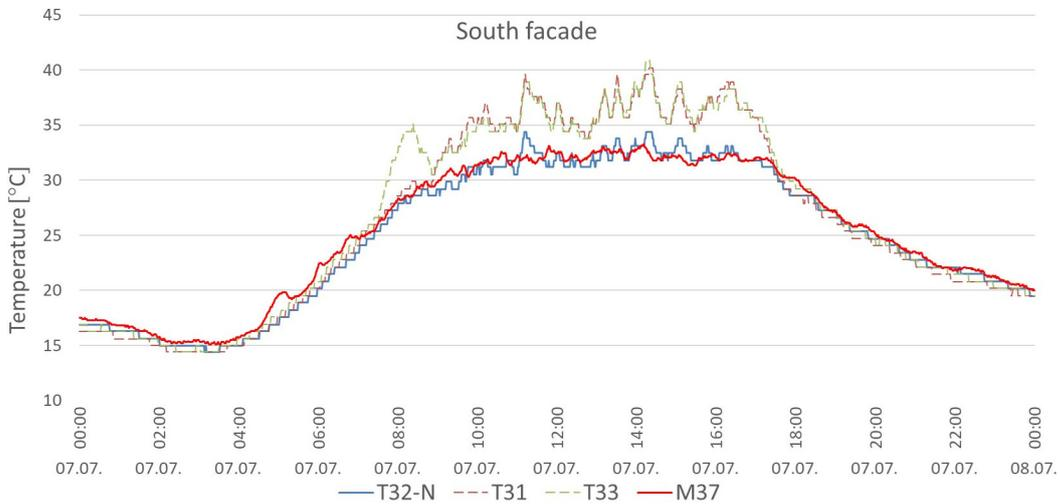
FIGURE 15. Daily temperature waveform recorded by FMS sensors on the south facade of the Research Centre building during 7 July 2021.
