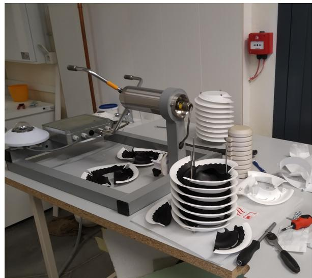
FIGURE 7. Installation and replacement of the new type of shield.
