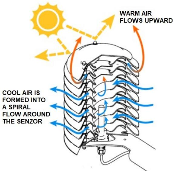
FIGURE 4. Illustration of airflow in the new shield [9].
