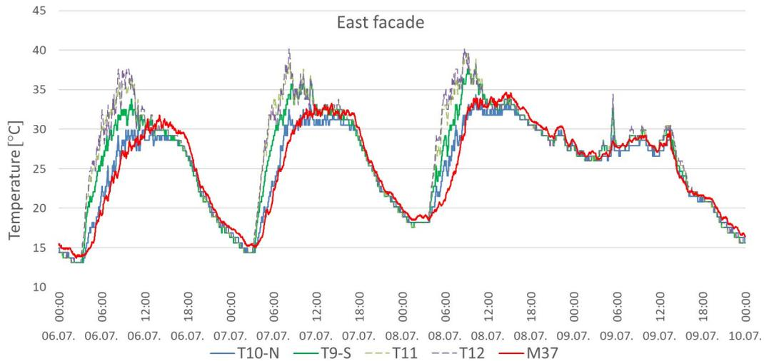
FIGURE 12. Temperature recorded at the FMS sensors on the east facade of the Research Centre building during 6 July 2021 to 9 July 2021.
