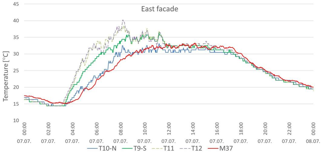
FIGURE 14. Daily temperature waveform recorded by FMS sensors on the east facade of the Research Centre building during 7 July 2021.
