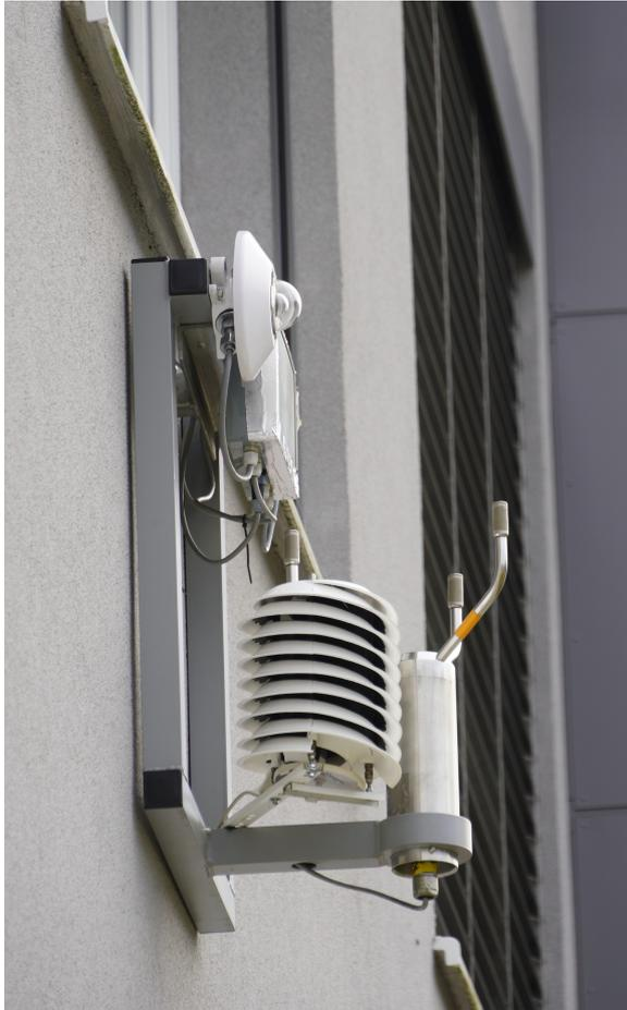
FIGURE 8. FMS with the new type of shield on the facade.
