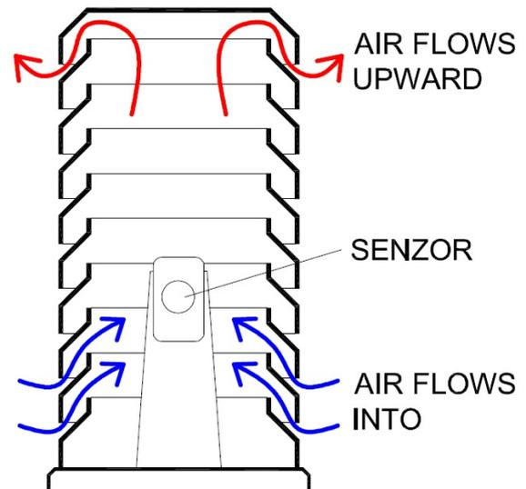
FIGURE 3. Illustration of airflow in the old shield.
