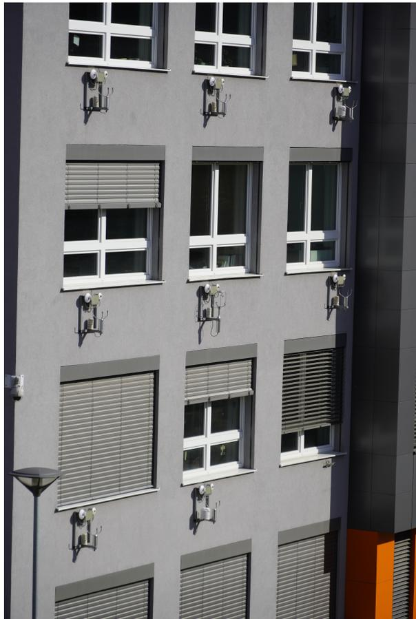
FIGURE 2. Meteo-stations located on the west facade of the Research Centre.
