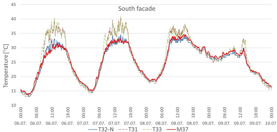
FIGURE 13. Temperature recorded at the FMS sensors on the south facade of the Research Centre building during 6 July 2021 to 9 July 2021.
