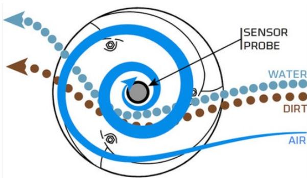
FIGURE 5. Schematic illustration of the eddy flow in the shield [9].
