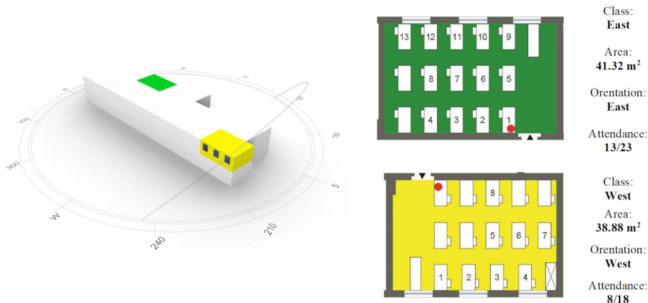
FIGURE 1. School building with sun path for the considered class period (November 16<sup>th</sup>–18<sup>th</sup>), classrooms configurations and position of nEMoS devices (in red) during the campaign.
