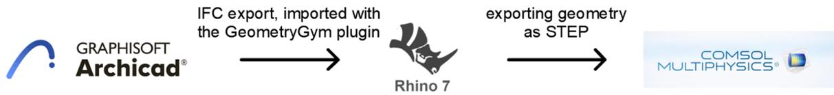
FIGURE 2. Open BIM workflow based on Archicad.
