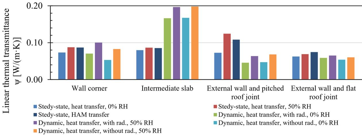
FIGURE 3. Linear thermal transmittance of construction joints under different modelling conditions.
