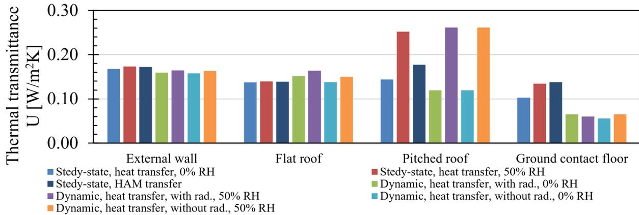
FIGURE 2. Thermal transmittance of the building envelope under different modelling conditions.
