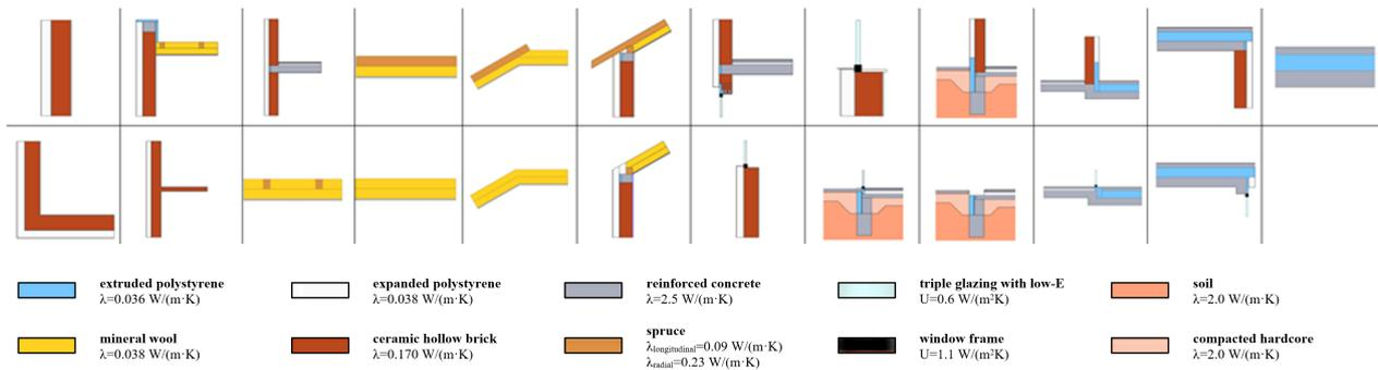
FIGURE 1. Analysed building construction joints of the examined building.
