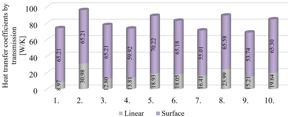
FIGURE 4. Comparison of heat transfer coefficients: 1) simplified calculation, 2) MSZ EN ISO 14683, 3) Thermal bridge catalogue, 4) steady-state and 0% RH, 5) steady-state and 50% RH, 6) steady-state HAM, 7) dynamic, with effect of radiation and 0% RH, 8) dynamic with solar radiation, 50% RH, 9) dynamic without solar radiation and 0% RH, 10) dynamic, without solar radiation and 50% RH.
