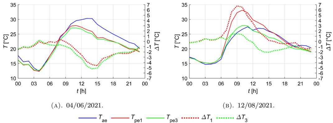
FIGURE 5. Surface temperature of plants  $T_{pe}$  compared with ambient air temperature  $T_{ae}$  in two selected clear sky days.
