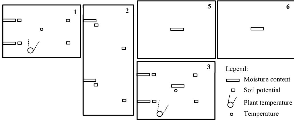
FIGURE 3. Position of sensors in test samples (external view on test samples – since 08/2021).
