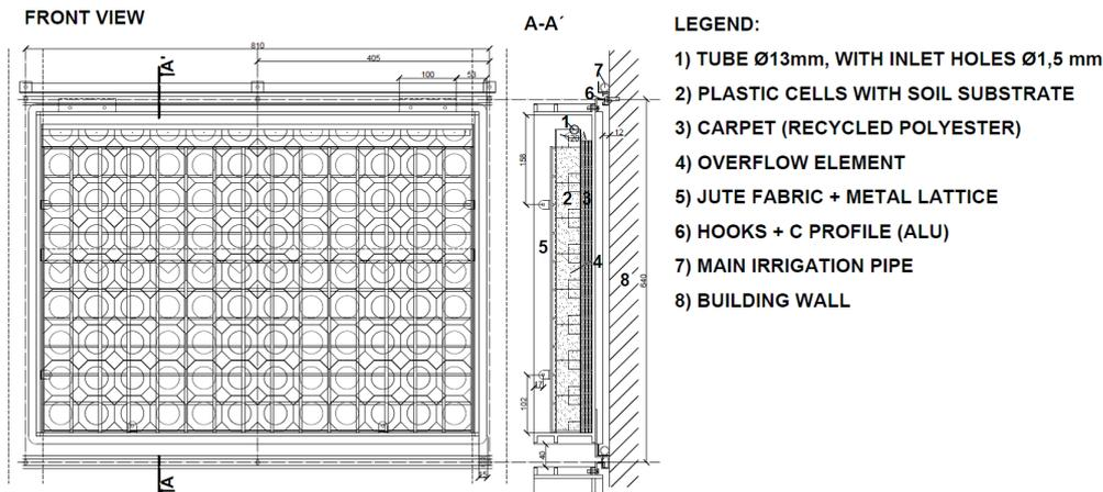
FIGURE 2. Technical drawing of test sample nr. 3.
