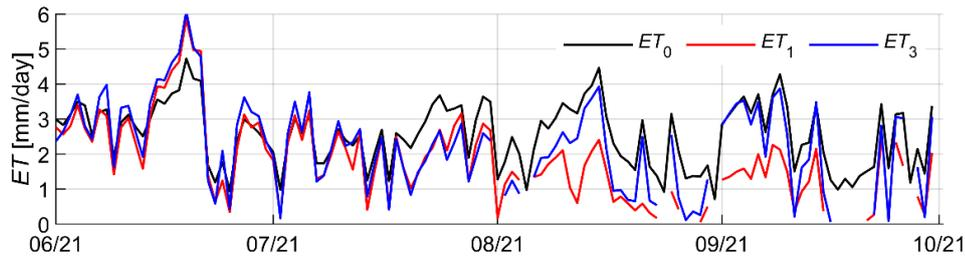
FIGURE 7. Evapotranspiration of test samples compared with reference evapotranspiration.
